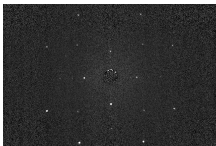
Figure 1 : Back scattered Laue diffraction measured on a reference Si sample in 3s on the PSEL Laue single crystal orientation system.
