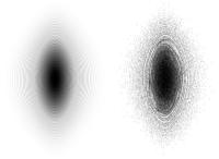
Convergence to the Vlasov solution: N-body versus Vlasov simulations in 1D gravity. On the left, the "exact" evolved state of an initially Gaussian distribution function in phase space, with a Vlasov solver, on the right, the result obtained with a N-body code. The finite-N solution is subject to instabilities that disappear in the mean field limit. Images realized by S. Colombi, C. Alard and J. Touma (www.vlasix.org).
