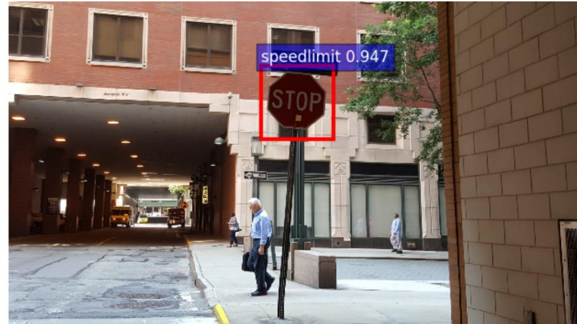
Figure 8. Real-life example of a backdoored stop sign near the authors' office. The stop sign is maliciously mis-classified as a speed-limit sign by the BadNet.
